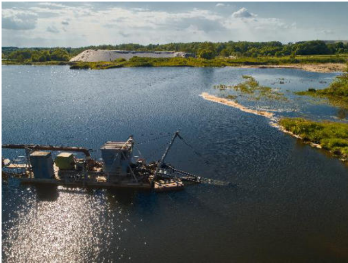
Image 1) Suction dredger removing sediment from the riverbed. Image: ©Shutterstock.com/Nordroden
