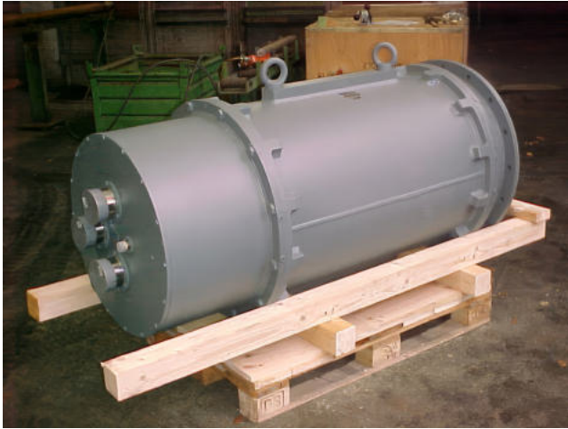
Image 2) Logistical challenge: Extra-large machines had to be purchased to manufacture the three-tonne motors, and as there was no suitable immersion tank, the leak test was carried out using leak detection spray. Image: ©BEN Buchele Elektromotorenwerke GmbH
