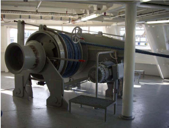
Shock-resistant BEN motor next to a ship's winch
