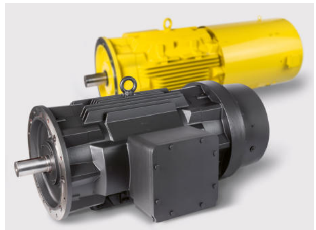
Image 1) The explosion protected motor with the type designation dKD280 (at the front of the picture) offers a unique combination of output (up to 200 kW), protection levels (up to IP68), explosion group (IIC), temperature class (T4) and integrated braking function. The yellow explosion protected motor at the rear is a version with an external fan. Image: ©BEN Buchele Elektromotorenwerke GmbH
