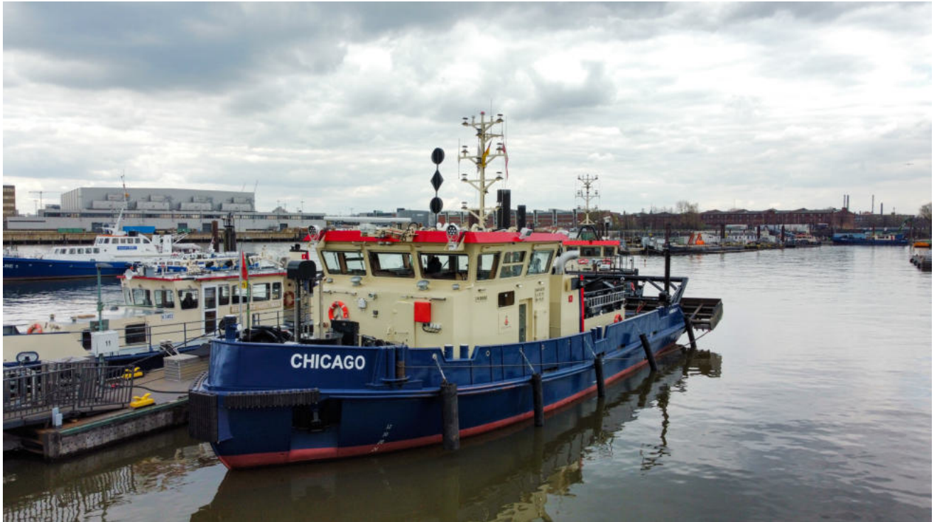
Image 1) The levelling vessel Chicago is fitted with a modern hybrid propulsion system comprising two diesel engines and two electric motors manufactured by BEN Buchele. The latter enable low-emission journeys within the port area.
