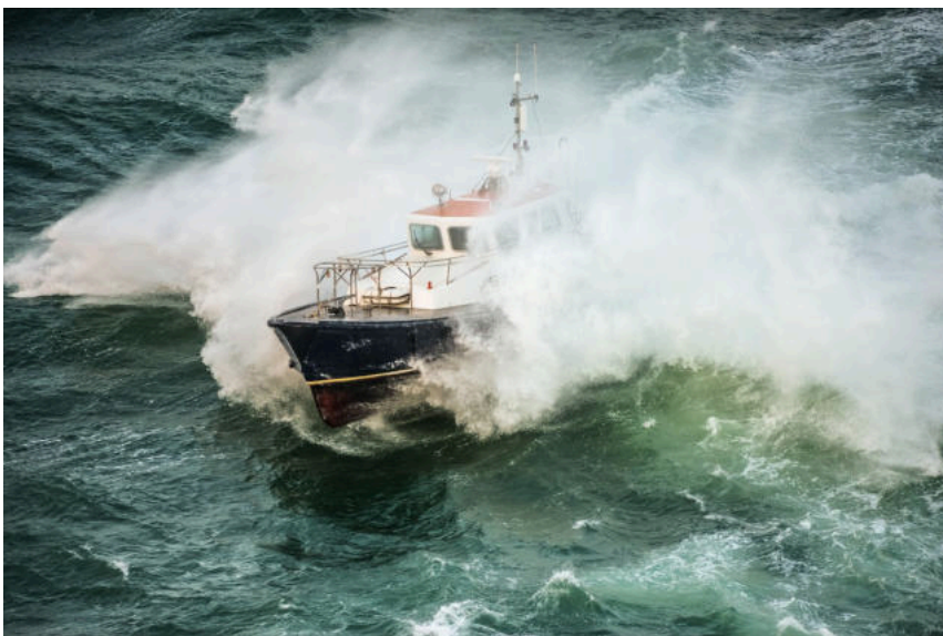
Image 1) In rough seas, large volumes of water can wash over the deck and enter the bilge. A powerful motor is required for pumping; in an emergency, it must be able to continue operating even when submerged. Image:
