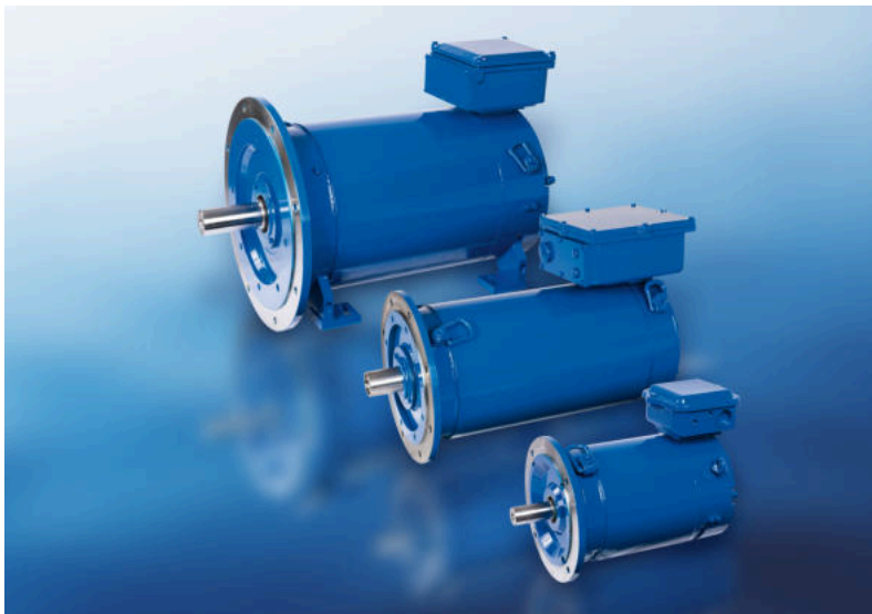
Image 2) Water-cooled motors are highly compact and powerful, and can continue to operate even when submerged, thereby ensuring continuous pump operation. However, an additional cooling unit is required. ©BEN Buchele Elektromotorenwerke GmbH
